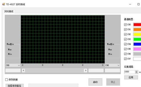
(1) The highest end of the curve interface corresponds to the upper range limit, and the lowest end of the curve interface corresponds to the lower range limit;
