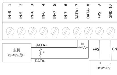
Input signal wiring diagram:
