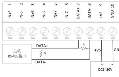
Enter the signal wiring diagram:
