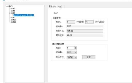
3、 The TD-4117 page is used to view the measured values of the module, configure the parameters, and modify the configuration parameters
